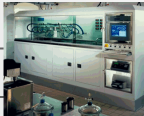
Multipass Test Stands with online Particle-Counting
