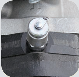
Triple sample access ports for in-operation fuel sampling
