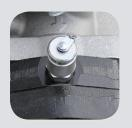
Twin sample access ports for in-operation oil sampling
