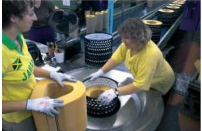
Inserting the filter bellows in the housing
