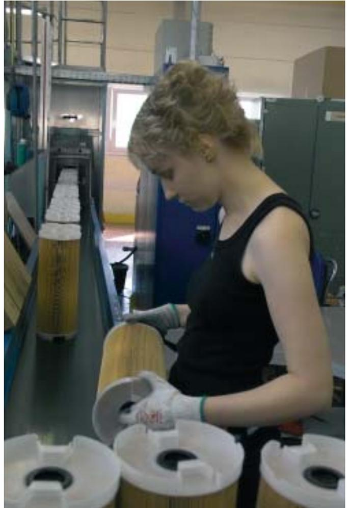
At the end of the production process a visual inspection ensures that only perfectly produced filters are delivered to the customer.
