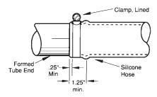
Initial torque on lined hose clamp should be 40 in·lb. If retorquing is required, limit to 20 in·lb.
